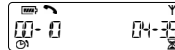
Figure 4. The elapsed call time (left) and approximate remaining talk time (right) appear when a call is in progress.
