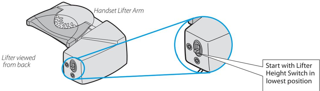
2. While wearing your headset, slide the Handset Lifter Arm under the handset until the lifter base touches the side of the phone.
