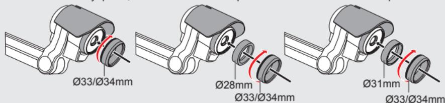
4. Mount the microscope adapter onto the Lens.
