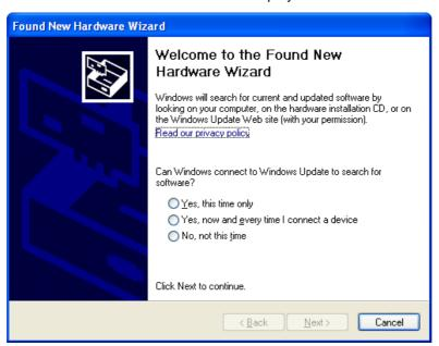
**NOTE:** If this wizard is not displayed, reconnect the USB cable between your computer and printer. The Hardware Wizard will display when the printer is properly connected.
