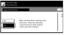
**5** To insert a cover page, press [Copy on front cvr] ([Copy on front cov.]).
