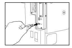
2 Connect the other side of the printer cable to the USB interface of the computer.
