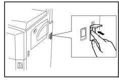
2 Connect the network cable to the network interface connector located on the rear right of this machine.
