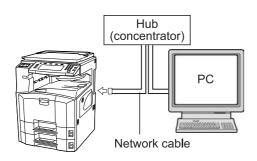
**1** Connect a network cable (100Base-TX, 10Base-T or the like) to the printer.
