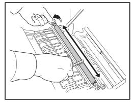
17 After completing the cleaning, replace the cleaning brush and close left cover 1.
