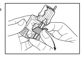
Insert the staple holder into the slot of the staple unit again.
