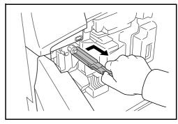
Take the grid cleaner provided out of its bag and remove the cap.
