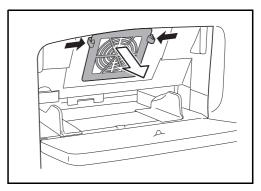
Remove dust from the filter using a vacuum cleaner or dry cloth.
