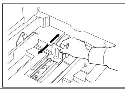
**NOTE:** Paper sizes are indicated on the cassettes. To change between inch size and metric size (A, B sizes), follow the steps below to adjust the size switch.
