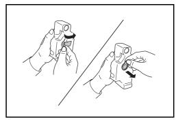
Fit the cap into the opening in the waste toner box and attach the sticker over the cap.
