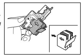
Insert the staple case fully as far as it will go. Pull to remove the paper tape wound on the staple case.
