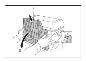
7 Turn the lever to lower the finisher process tray.
