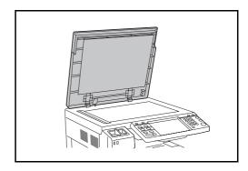
**NOTE:** If the optional document processor is installed, open the document processor. Before opening the document processor, be sure that there are no originals left on the original table or on the original eject table. Originals left on the original table or on the original eject table may fall off when the document processor is opened.
