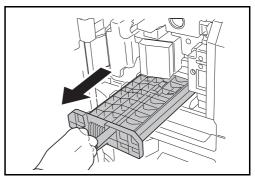
**7** Open paper feed unit cover (A3) and remove the jammed paper.
