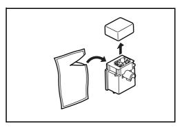
Align the grid cleaner with the notch and attach it to the machine.
