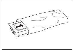
Unwrap a new toner container and hold the new toner container upright and tap the top of the container 5 or more times.
