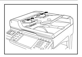
Place the originals. Put the side to be scanned (or the first side of two-sided originals) face-up. Slide the leading edge into the document processor as far as it will go. The original placement indicator will be lit.
