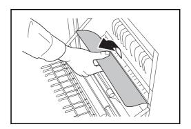
Lift up duplex unit and remove the jammed paper.
