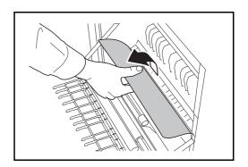
Lift up the duplex unit and remove the jammed paper.
