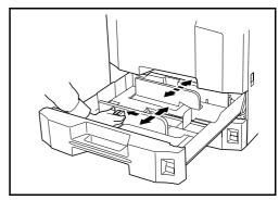
Using the paper length guide, 3 move the plate to fit the paper.
