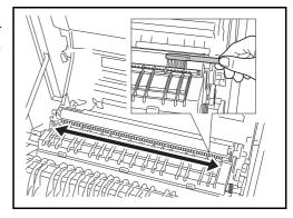
As shown in the figure, clean off any soiling on the transfer roller by moving the brush from side to side along the roller while rotating the roller by turning the gear at the left end of the roller.
