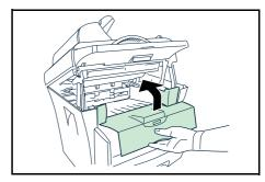
4 Lift the *Developer Unit* together with the *Toner Container* out of the printer.
