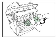
4 Using the green handles lift the *Drum Unit* out of the machine.
