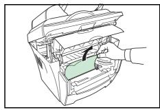
6 Return the *Drum Unit* to its position, aligning the guides at both ends with the slots in the machine.
