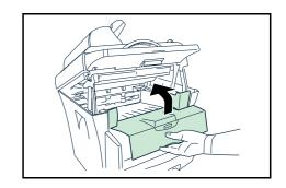
3 Lift the *Developer Unit* together with the *Toner Container* out of the printer.
