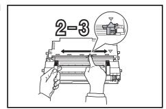
When cleaning is complete, return the *Drum Unit* to its position, aligning the guides at both ends with the slots in the machine.
