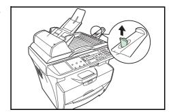
Arrange the originals in order and place them face up on the original table. Slide the leading edge of the originals securely into the document processor as far as they will go.
