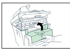
3 Lift the *Developer Unit* together with the *Toner Container* out of the printer.
