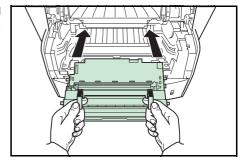
8 Insert the *Developer Unit* together with the *Toner Container*, back into the machine.
