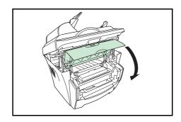
Olose the Scan Unit pushing the Lever.
