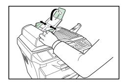
4 Pull the ejection extension when using A4.
