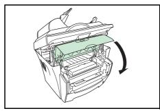
10 Close the Scan Unit pushing the Lever.
