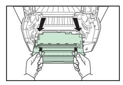
5 Place the *Drum Unit* flat on a clean, level surface.
