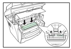
7 Turn Lock Lever A to the lock position.
