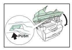
**IMPORTANT:** Take care not to place your fingers between the scan unit and the main body when the scan unit is closed.
