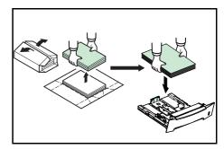
When you open a new package of paper, fan through the sheets to separate them slightly prior to loading. If the paper is curled or folded, straighten it before loading. Paper that is curled or folded may cause paper jams.
