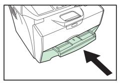
Adjust the paper width guides and slide the paper into the tray as far as it will go. The side to be printed should be face up.
