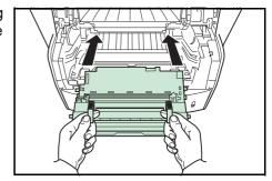
7 Insert the *Developer Unit* together with the *Toner Container*, back into the machine.
