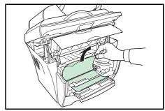
If it has not be fed as far as the metal registration roller, remove the paper from the *Manual Feed Tray* side.
