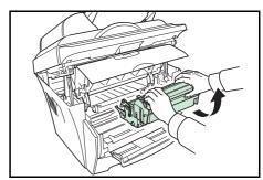
5 Using the green handles lift the *Drum Unit* out of the machine.
