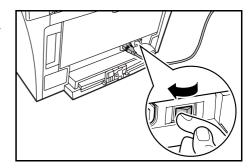
Connect the USB cable to the USB interface connector located at the rear side of the machine.
