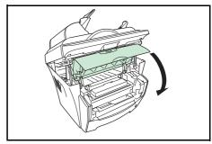
7 Close the Scan Unit pushing the Lever.
