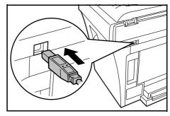
3 Connect the other end of the USB cable to the USB interface connector on your computer.
