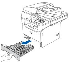
2 While pressing the blue paper guide release lever (1), slide the adjusters to fit the paper size. Check that the guides are firmly in the slots.
