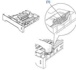
For Legal size paper, press the lever (1) located at the back of the tray and pull out the back of the paper tray. Move the tray lock button (2) to the lock position.
