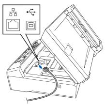
Carefully route the network cable through the trench and out the back of the machine. Then, connect the cable to your network.
