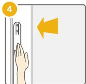
4. Press the metal brackets firmly against the board for best adhesion. Do this on the top and bottom of the system.
