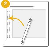
2. Holding template vertically and by the edges, determine placement. If you are installing the system on a whiteboard, make sure to leave 2 inches (5.08 cm) between the Engage System and the board frame.
