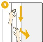
5. To remove the template, pull down and lift it out from beneath the Engage System.
