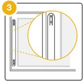
3. Place the template so that it is centered vertically on the board and parallel to the frame.
