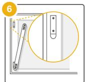
6. After the template is removed, confirm that the top and bottom brackets are firmly attached to the board, if necessary press down on them again. \*Note: 3M recommends waiting at least one hour for maximum adhesion.
