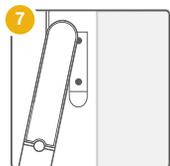
7. Align the brackets with the four holes on the back of the Engage System.
