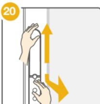
20. Lift the Engage system upward to release from brackets and pull away from surface to remove.
