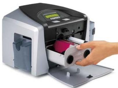
*The Fargo DTC400 Card Printer/Encoder is designed for easy operation and hassle-free maintenance. The SmartLoad Ribbon Cartridge combines a printer ribbon and card cleaning roller into one disposable or refillable unit. Just slide in the cartridge, close the door, and you're done. No feeding or tearing ribbon rolls, no fumbling with separate cleaning rollers.*
