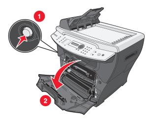
2 Pull on the handle to remove the print cartridge assembly.
