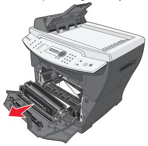
**Warning:** Do not leave the print cartridge assembly exposed to direct light for an extended period of time. Extended light exposure can cause print quality problems.
