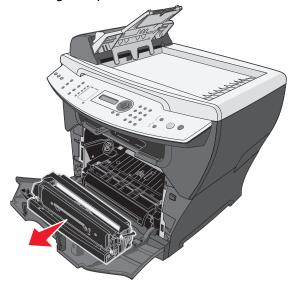
**3** Place the print cartridge assembly on a clean, dry surface.
