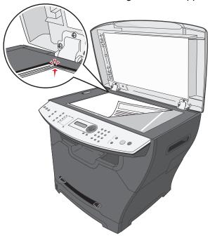
3 Close the top cover to avoid dark edges on the scanned image.
