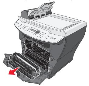
3 Place the print cartridge assembly on a flat, clean surface.
