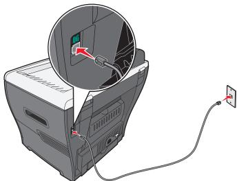
**3** Remove the protective plug from the EXT port of the MFP.
