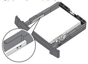
7 Squeeze and adjust the paper guides until they lightly touch the side of the stack of paper.
