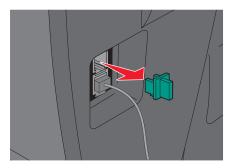
4 Connect the other telephone cord to a telephone, and then plug it into the EXT port in of the MFP.
