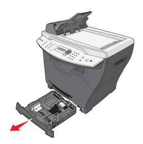
**3** Holding the tray on a stable surface, press the guide lock, and slide the rear guide until it locks at the paper length you want.
