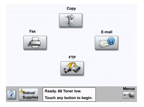
The MFP control panel alerts you once a supply item or maintenance is required. The Print status message bar at the bottom of the touch screen indicates if the MFP is Ready and lets you know if any supplies are low or empty. Touching Status / Supplies on the bottom of the touch screen will open the Status / Supplies screen where you can view the status of the various trays and other supply items.
