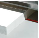
An optical cutting line indicates exact location of cut and helps to perfectly position trim marks.
