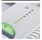
"ECC" (Electronic Capacity Control) indicator helps prevent paper jams by monitoring capacity levels during operation.
