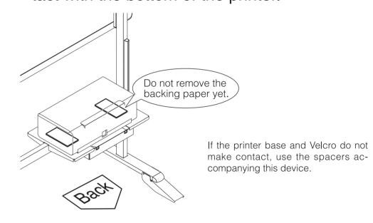
3 Attach the Velcro to prevent the printer falling.
