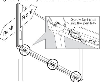
**7** Connect the screw holes on the pen tray to the screws for installing the pen tray.
