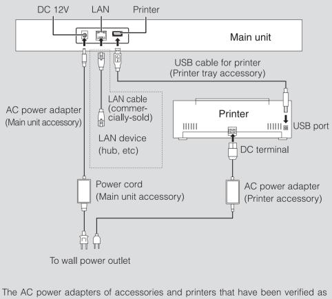
operable may differ from the ones shown in the wiring diagram (they may be of the built-in or mounted-on type).
