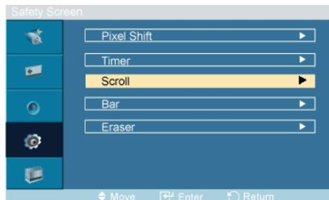
This function helps to remove after-images on the screen by moving all the pixels on the LCD according to a pattern.
