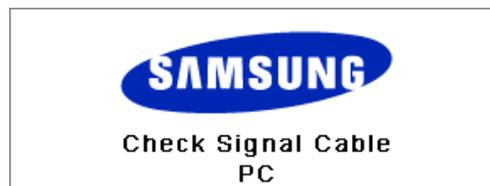
4. Turn off your LCD Display and reconnect the video cable; and then turn on both your computer and the LCD Display
