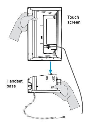
**B** Fasten the two units together. The screws are pre-mounted in the handset base.
