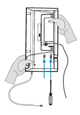
Connect the handset to the handset base, and connect the handset cable.
