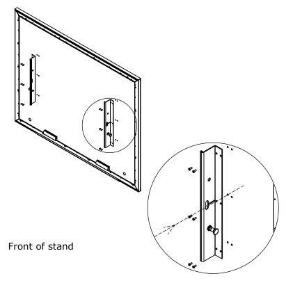
5. Attach brackets as shown with (12) 8#-32 screws. (Do not over tighten.)
