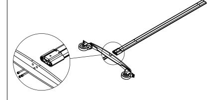
1. Attach connector to leg using (3) 1/4-20 flat bolts. Flip leg and attach base to leg using (3) 1/4-20 bolts. Tighten all (12) bolts.
