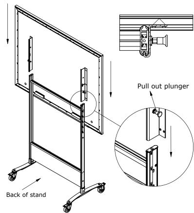
6. Position adjustable brackets into slots of uprights. Pull out plunger and position at lowest adjustment hole. (Two people required.)
