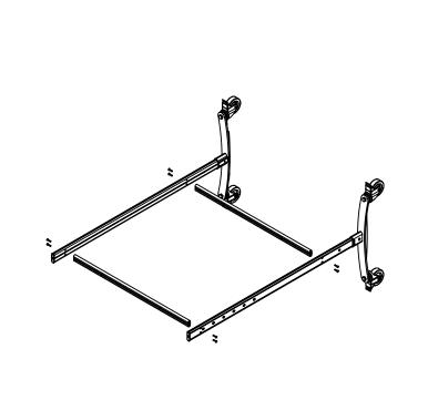
2. Attach cross members to uprights using (8) 10-24 screws. (Do not completely tighten until end of Step 3.)
