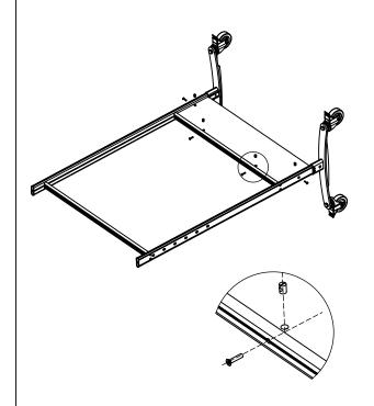
3. Insert (4) cross dowels into holes of bottom support panel. Be sure holes in cross dowel facing toward outer hole on panel. Position panel as shown and attach with (4) M6x35 screws. Tighten all (12)screws and stand upright.
